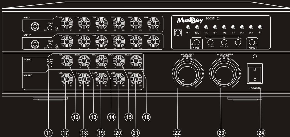
11. ST/MO (Stereo/Mono) - Use this button to switch between the two echo output modes, STEREO and MONO.
